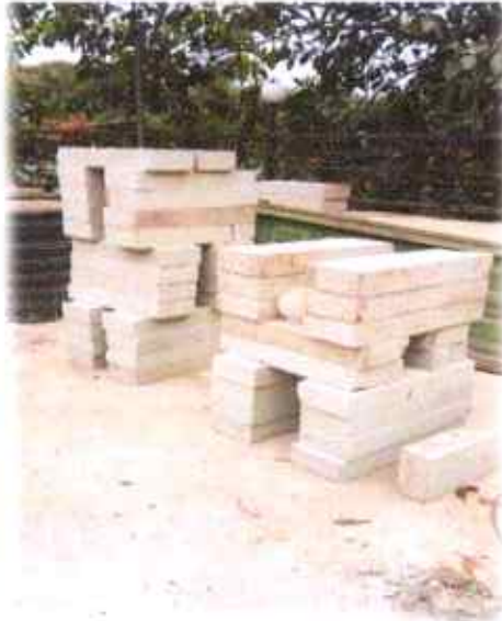
AERATED CONCRETE BLOCKS USED IN CONSTRUCTION AS LIGHTWEIGHT.
