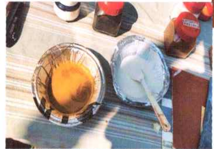
3. CREATION OF BINDER BY PROTEIN AND LIME MIX.
