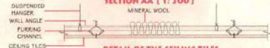
DETAIL OF THE CEILING TILES
