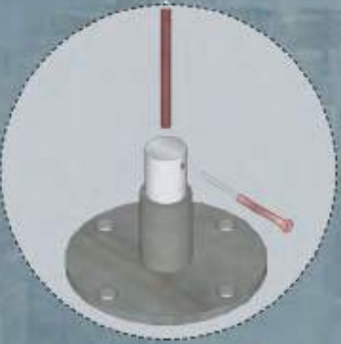
To stabilize the panels steel rod is inserted in footing plate which is fixed by screw.
